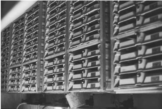
Figure 5. Heath Vertical egg-incubation system.
