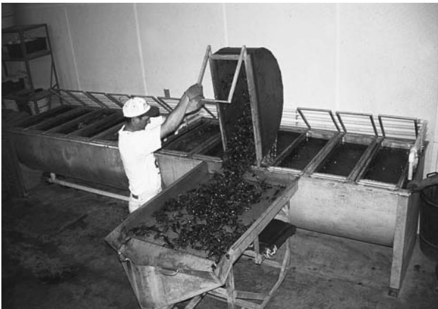
Figure 13. Nonearthen raceways with suspended baskets are effective and efficient purging systems when adequate water exchange and supplemental aeration are used.
