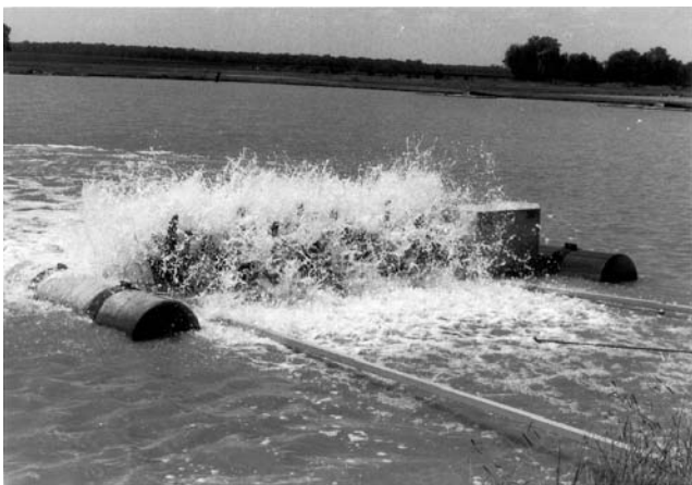
Figure 7. An electric paddlewheel aerator.
