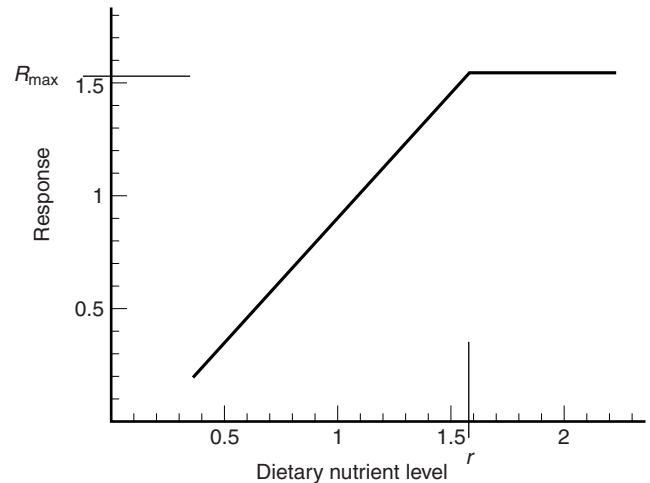
Figure 2. The relationship of physiological response to the concentration of a required nutrient, using the broken line model. The requirement ( r ) is determined to be the nutrient concentration corresponding to the intersection of the two parts of the line.
