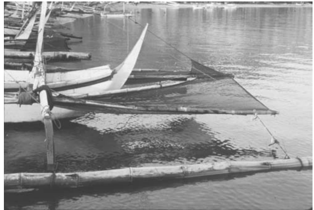
Figure 1. Boat equipped with fry collection gear.
